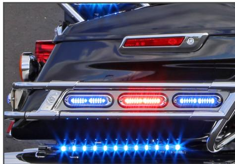
**NEW Side Crash Bar Mounting Bracket Kit/Side (Saddle Bag) Crash Bar Mounting Bracket Kit** allows for easy mounting of three ION T-Series or surface mount ION lightheads. Durable stainless steel construction.
